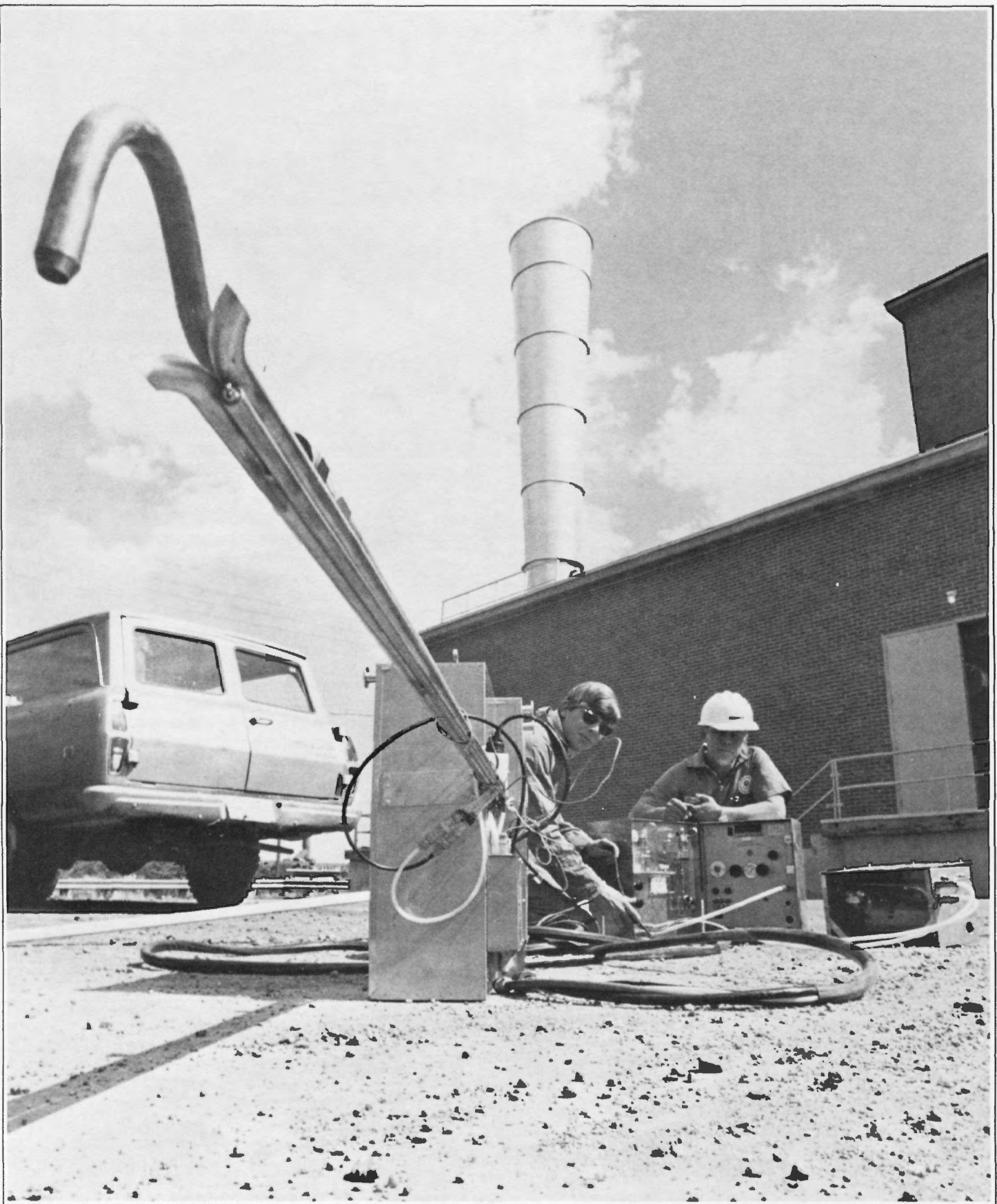
Paul R. De Percin and George Stone (wearing hard hat), set up equipment to sample fumes in smokestack behind them. The sensor will be raised to the smokestack where it will monitor the stack airflow.
